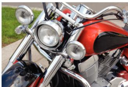
Figure 1 Chromium-plated objects look very shiny and attractive. The chromium layer does not corrode away so it protects the steel beneath from rusting.
