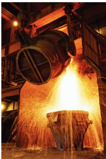
Figure 1 The iron which has just come out of a blast furnace contains about 96% iron. The main impurity is carbon.
