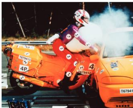
Figure 1 Crash-test dummies are used to gauge the best volume of gas to cushion the effects of a collision. A sensor detects the sudden deceleration and completes an electrical circuit to ignite the chemicals in the air-bag.
