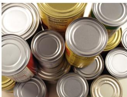
Figure 2 So-called 'tin' cans actually contain very little tin. The layer on the steel can be only a few thousandths of a millimetre thick! The tin keeps air and water away from the iron in steel and stops it rusting – at least until the tin gets scratched! Tin is quite a soft metal, unlike chromium.
