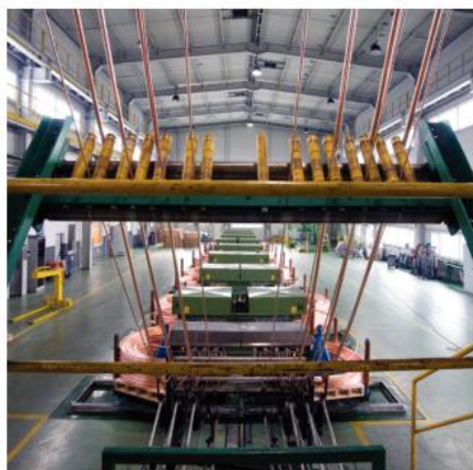
Figure 1 Drawing copper out into wires depends on being able to make the layers of metal atoms slide easily over each other, without breaking the metal
