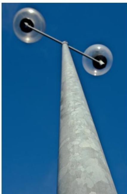
Figure 3 Metal crystals, such as the zinc ones shown on this galvanised lamp post, give us evidence that metals are made up of atoms arranged in regular patterns
