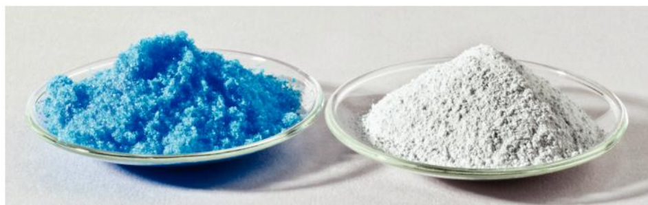
Figure 2 Hydrated copper(II) sulfate and white anhydrous copper(II) sulfate
