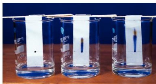
Figure 2 Black ink can be separated out into its different colours on a chromatogram
