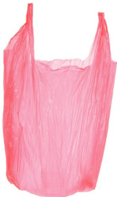
Figure 1 The forces between the molecules in poly(ethene) are relatively weak as there are no strong covalent bonds (cross links) between the molecules. This means that this plastic softens fairly easily when heated.
