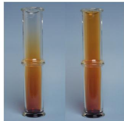
Figure 2 Bromine vapour diffuses and mixes thoroughly with the air
