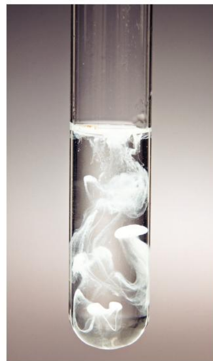
Figure 3 The white precipitate of barium sulfate forming
