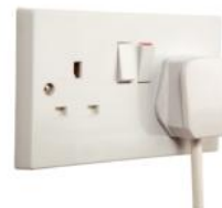
Figure 4 Electrical sockets are made out of thermosetting polymers. If the plug or wires get hot, the socket will not soften.
