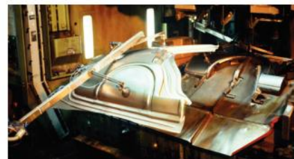
Figure 2 Low carbon steel called mild steel is easily pressed into shapes
