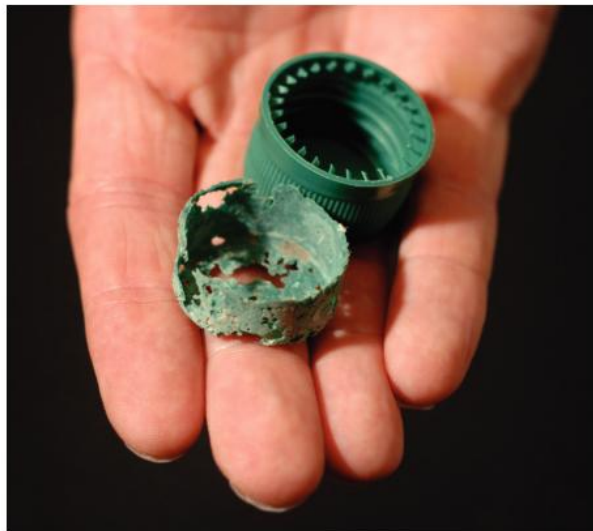
Figure 2 The breakdown of a biodegradable polymer. PLA can be designed to break down in a few months.
