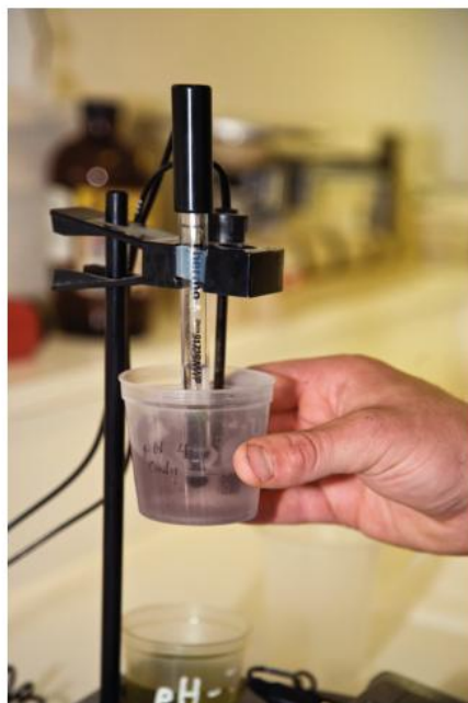
Figure 2 Testing the pH of a solution using a pH sensor
