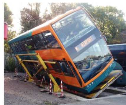
Figure 4 A toppling test
