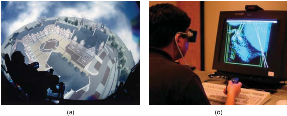
Figure 6 (a) Bird's-eye view from the flight chair in the Hemispherium™; (b) Fishtank VR display.
