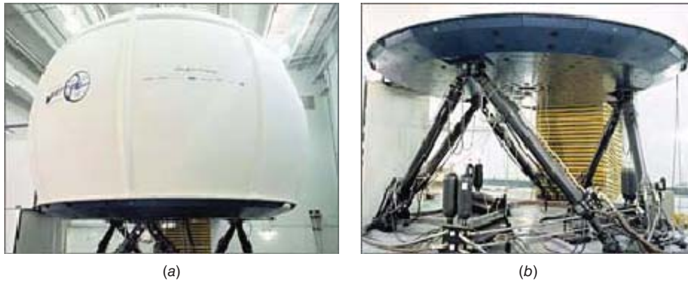
Figure 25 VIRTTEX driving simulator.
