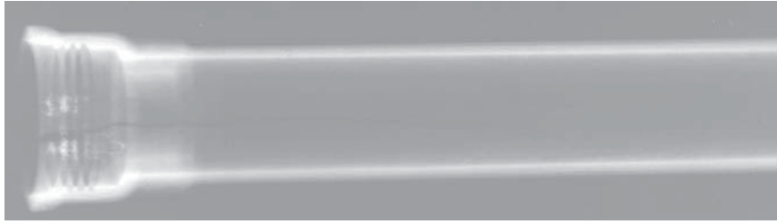
Figure 7 Radiograph of crack in end of aluminum tubing.
