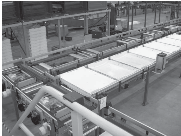
Figure 18 EBS elements, here storing a line of empty totes.
