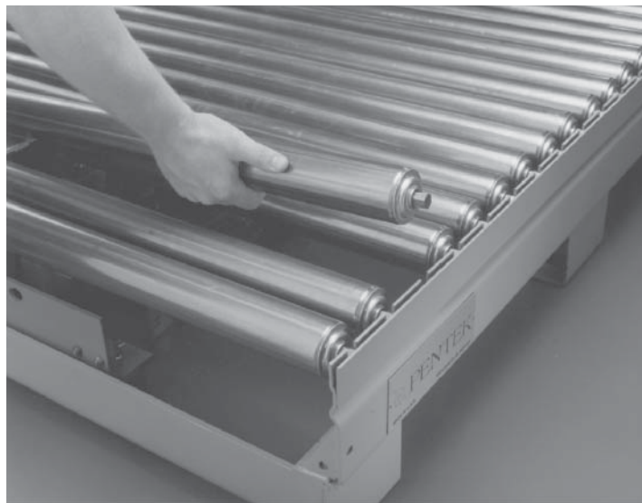
Figure 1 Gravity roller conveyor. Courtesy of Pentek.
