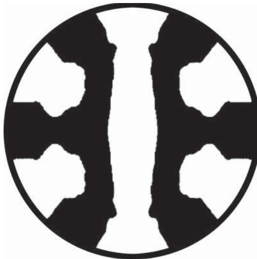
Figure 16 Hemispherical shading pattern for Delta-T BF3 irradiance sensor.
