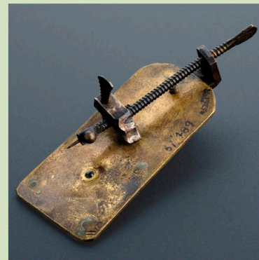
This is a replica of the first microscope by van Leeuwenhoek, who achieved up to 300 times magnification using a single lens.
