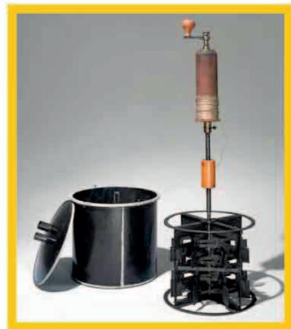
**In Joule's experiment**, a falling weight drove a paddle that turned inside a bucket of water. The energy of the movement was changed into heat.
