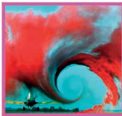
**Here, turbulence** forms at the tip of a vortex left in the wake of an aircraft’s wing. Study of the critical point beyond which a system creates turbulence was key to the development of chaos theory.
