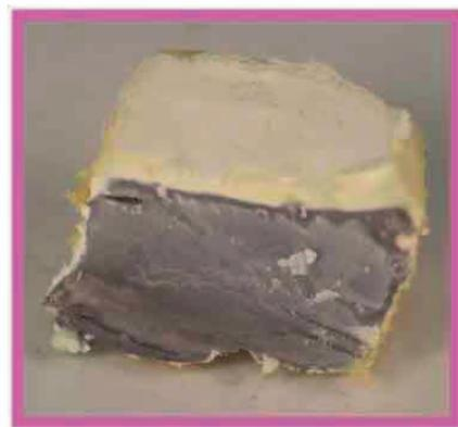
**The six alkali metals** are all soft, highly reactive metals. The outer layer of this lump of pure sodium has reacted with the oxygen in the air to give it a coating of sodium oxide.
