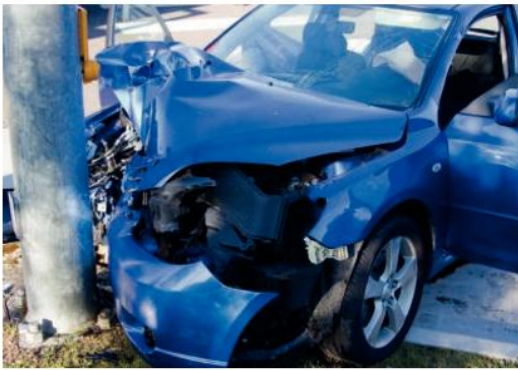
This car has crashed into a steel pole. Nobody was hurt because the front part of the car crumpled and absorbed the kinetic energy of the car.
