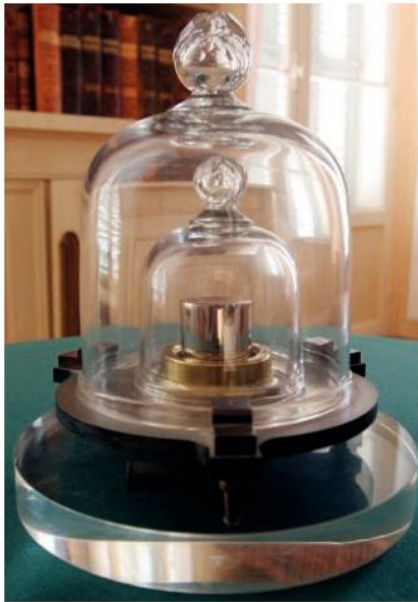
This piece of material is a copy of the 'International Prototype Kilogram' and it has a mass of exactly 1 kg
