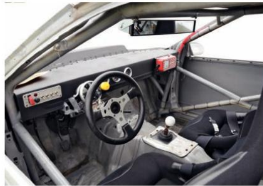
The inside of this racing car has extra steel tubing to create a strong protective cage for the driver. Normal cars are designed to have strong passenger areas too.
