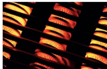
These coils of wire in an 'electric fire' are giving out so much heat energy they are glowing red hot!
