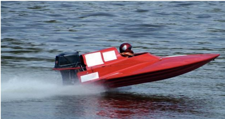
This fast boat skims across the top surface of the water, reducing the water resistance
