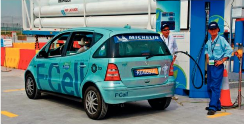
An experimental hydrogen fuel cell car being refuelled; this is much quicker than charging the battery in a normal electric car
