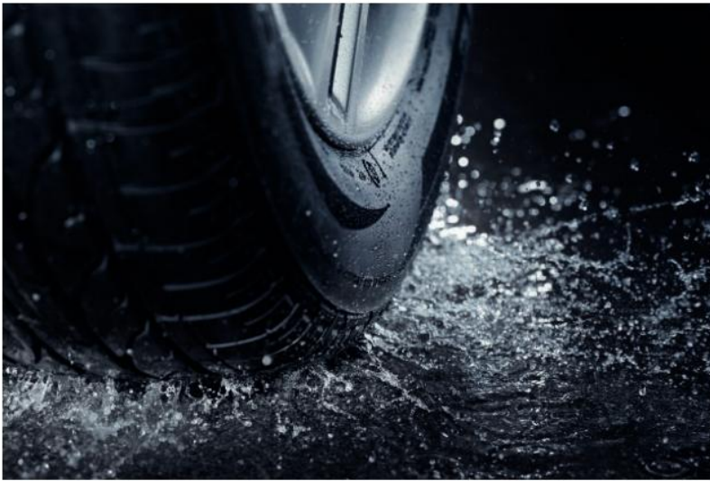
This rubber car tyre has good grip on the road and the tread pattern helps to push the water (a lubricant) out of the way
