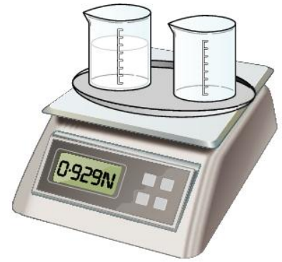
This top pan balance is being used to measure the weight of a small sample
