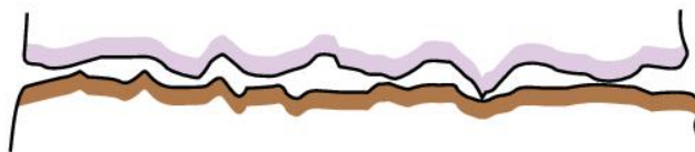
The rough parts of the surfaces catch on each other and prevent movement
