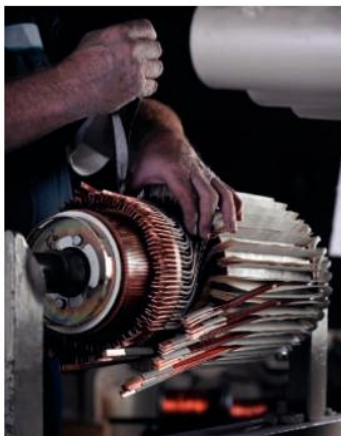
An electrical motor converts electrical energy into kinetic energy. This large motor is used in elevators.
