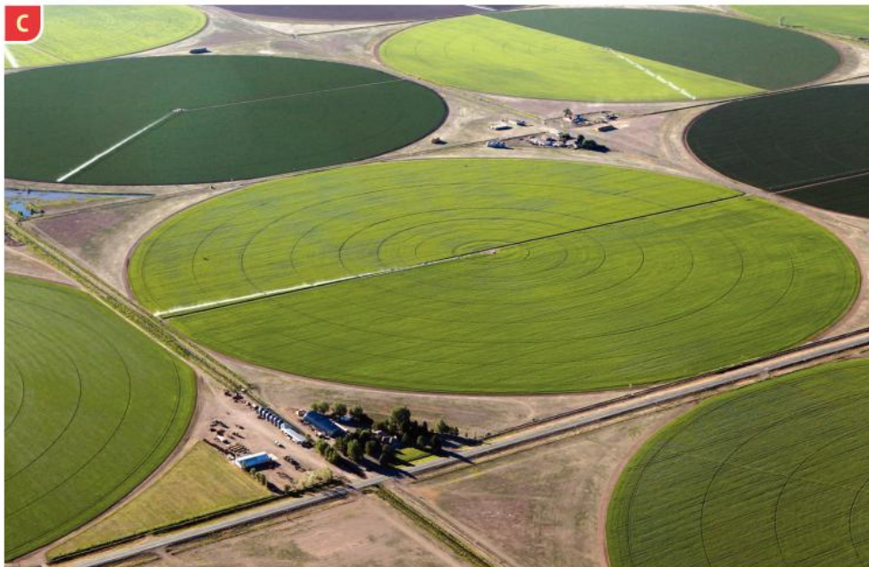
▲ Where Doug and Brad live. The green circles are crops. Giant arms rotate like a clock hand, sprinkling the crops with water from the Ogallala. Look how long the sprinkler arms are, compared with the buildings.
