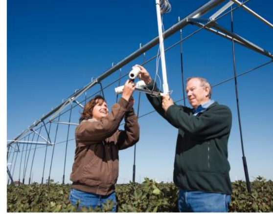
▲ Fitting sensors to sprinklers in Texas, to help the Ogallala. They measure leaf temperature, and tell the sprinklers when to turn on.
