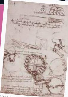
This Leonardo drawing shows a weapon for hurling stones—a bombard—powered by a water wheel.
