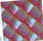
Despite their strength, Kevlar fibers are flexible enough to be woven into labric. They are also used in ropes.
